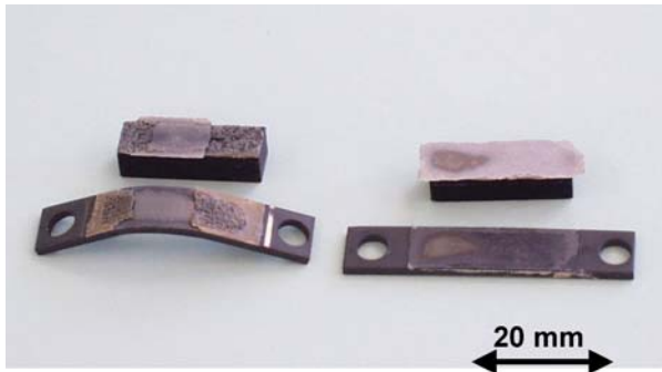
Figure 6 Fracture behaviour of glass braze joints for different surface preparation state of the metallic substrate at the end of the bending test. Right: Mo plate in as-delivered state (smooth surface), left: Mo plate with sand blasted surface.
